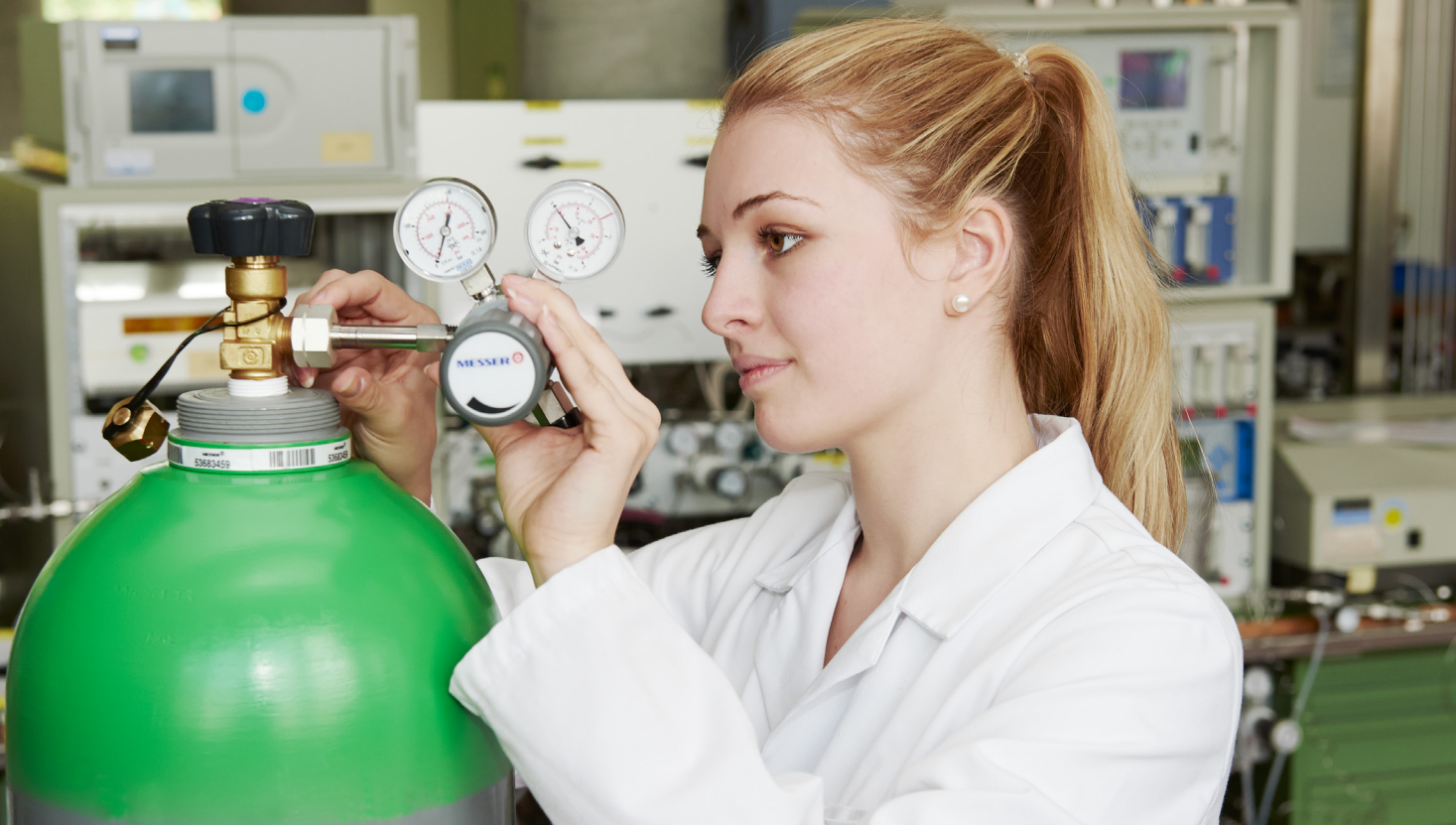
Individual cylinder at the point of use with cylinder pressure regulator
